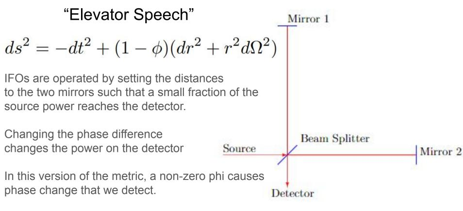
This detection is at the input light's reference frequency  $c/\lambda$  and also in sidebands.
