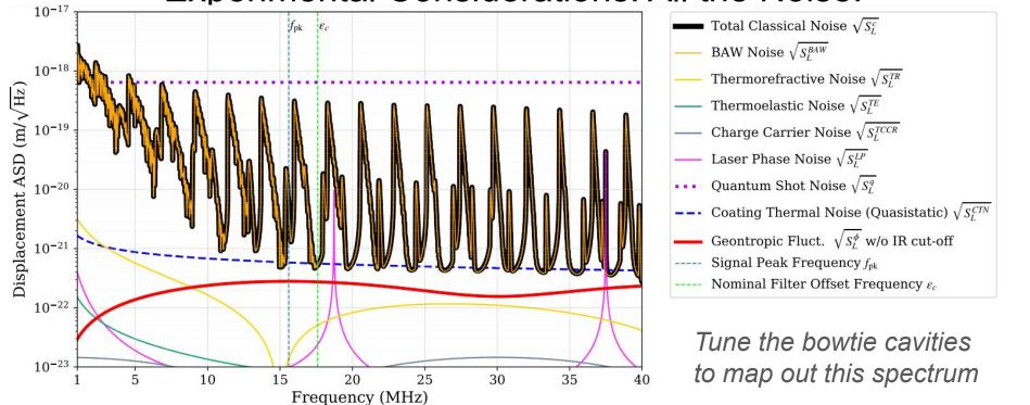
Mirrors are not perfect: the substrate is a drum; coatings have thermal noise
